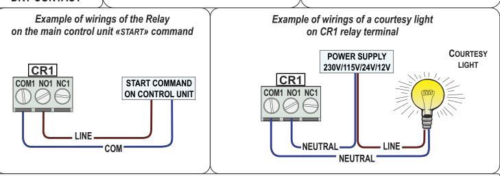
\* Each relay terminal supports a maximum load of 3A and 250Vac
