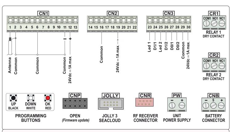
\* All the 24V inputs support a maximum load of 1A referred to the sum of the loads of all 24V accessories connected, including the absorption of the receiver on board (30 mA)
